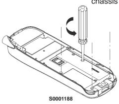
Then unscrew two UI module screws.
